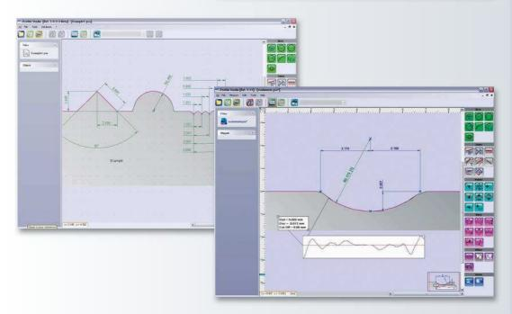
Fast. easy setting and evaluation of achieved results. Each relevant dimension can be input upon recognition of the part geometry feature (a point, straight line or arc of circle). Both the rotation and symmetry of the profile being checked let it be conveniently aligned.
