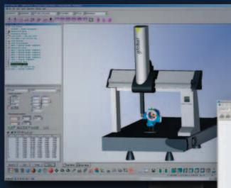
**PC-DMIS software** takes full advantage of Global scanning capability. In the example shown, the machined flange surface is being scanned for flatness; PC-DMIS allows for the specification of scan paths, shown as the yellow curvilinear line below.
