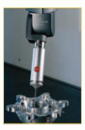
The LSP-X1 leverages world-renowned Leitz scanning technology in a compact continuous contact sensor. Mounted on a TESASTAR-m or TESASTAR-sm indexable motorized probe head, the LSP-X1 features the ultimate in high speed scanning measurement flexibility, with outstanding performance in both touch trigger and scanning modes.
