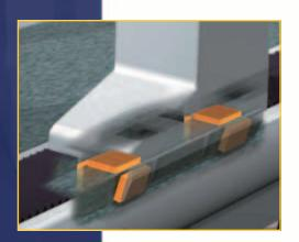
Wrap-around air bearings on precisely machined dovetail guideways provide optimum measuring repeatability and long term system stability. Easy-maintenance, pre-loaded Belleville springs assure constant force over the machine's entire travel distance.
