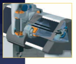
Steel reinforced closed-loop belt drive is precision engineered with elliptical tooth profile to reduce machine vibration at high scanning speeds.
